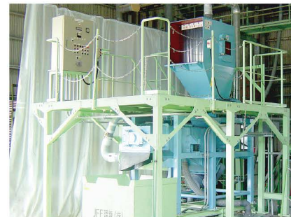
Beverage containers Bottles crushing equipment
